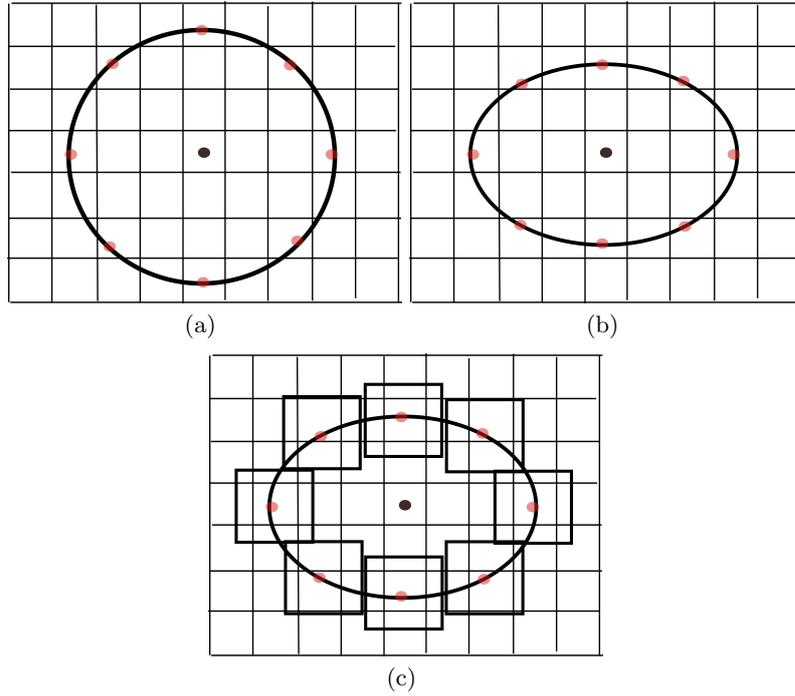
**Fig. 3.** LBP pattern for (a)  $LBP^{P,R=3}(x_c, y_c)$ , (b)  $ELBP^{P,R_1=3,R_2=2}(x_c, y_c)$  (c)  $M-ELBP^{P,R_1=3,R_2=2}(x_c, y_c)$  where  $P=8$ .
